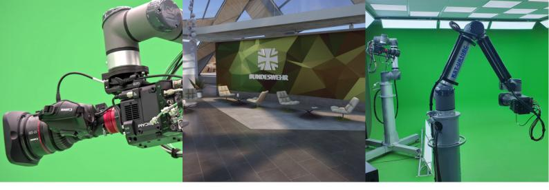
Work in the studio begun by setting up a green area measuring around 6 x 6 metres. Executed in the VR-studio colour RealGreen, the L-shaped cyclorama construction in combination with the extremely homogeneous lighting of KST's 5900k VR light set create the basis for establishing a successful VR workflow.
